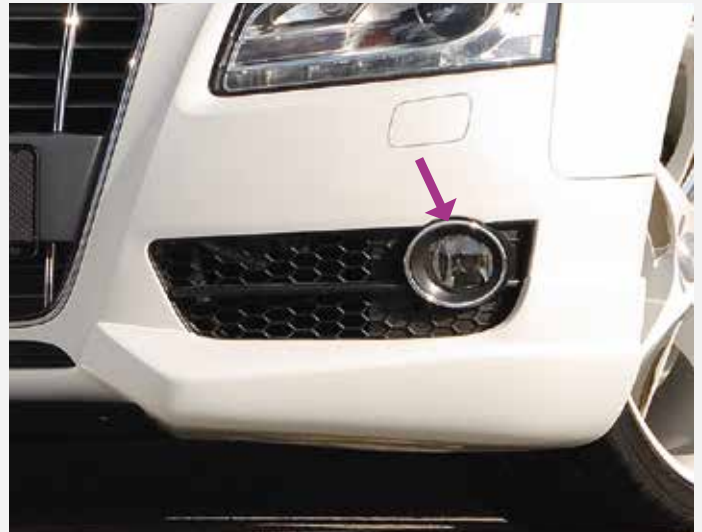
The cover of the fog lights for non S-Line has three bars.
