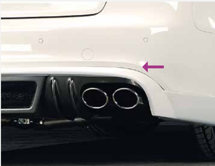
On S-Line, there is a light edge above the rear insert.
