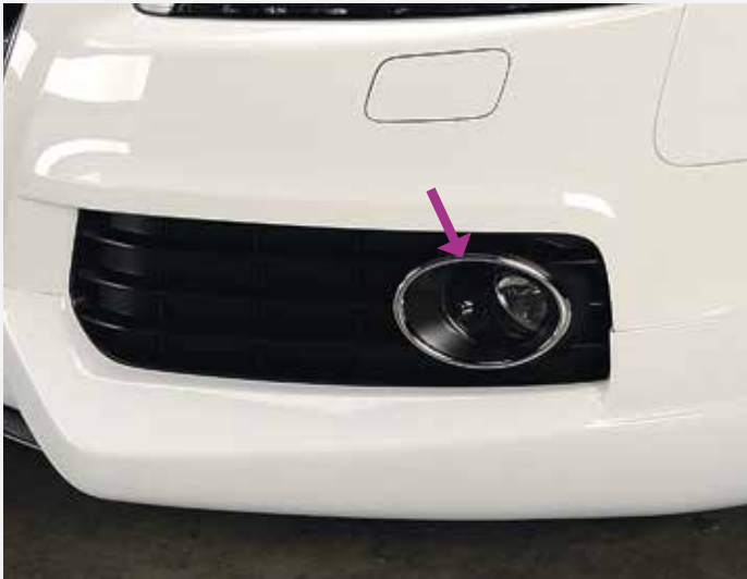
S-Line has two bars in the fog light cover.
