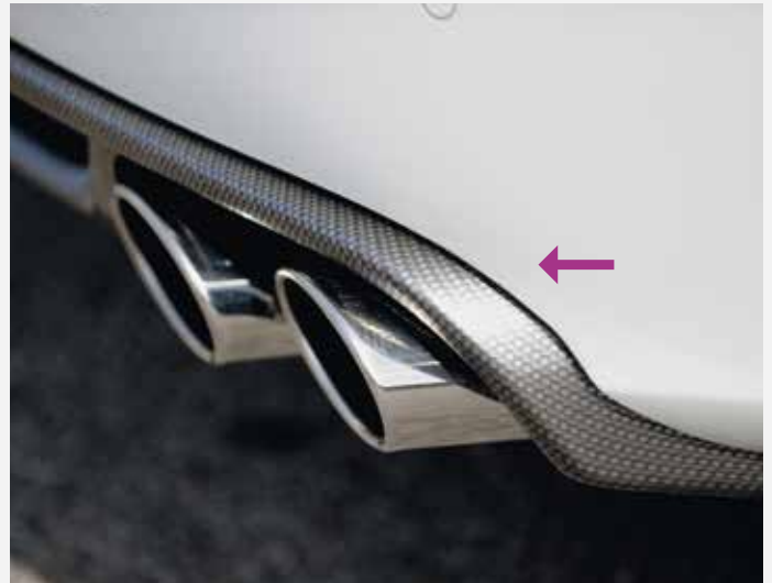
With non S-Line there is no light edge above the rear insert.
