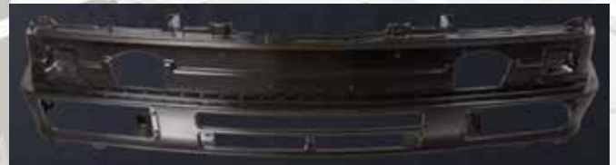
Wind deflector, required for vehicles before 09.87
