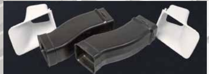
Air nozzles (white) and brake air ducts, required on vehicles before 09.87
