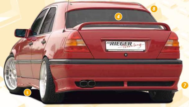
In the rear wing without brake light, an adapter plate is mounted instead of the lamp. We recommend the use of a sports rear muffler, with the standard rear muffler it can lead to merges on the rear skirt.
