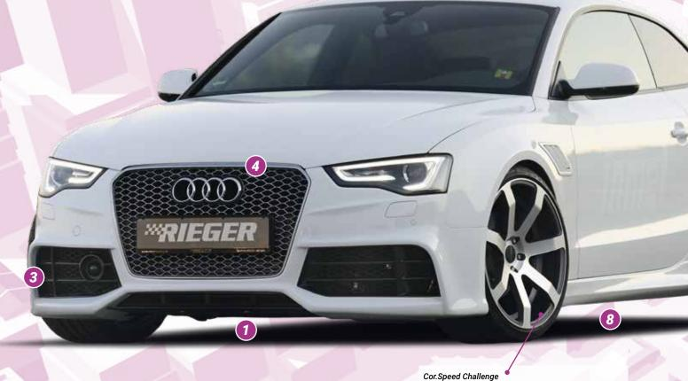
VA 10,0Jx20 ET 45 with 265/30-20 + 20 mm Spacer HA 10,0Jx20 ET 45 with 265/30-20 + 25 mm Spacer
